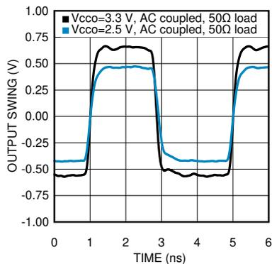
**Figure 7-9. LVCMOS Output Swing at 250 MHz**
