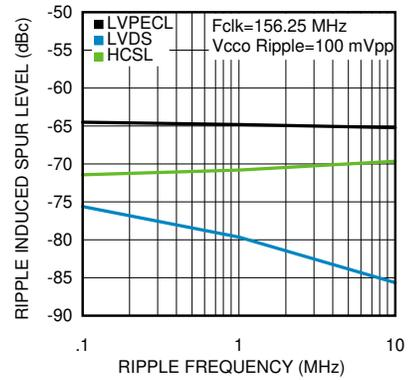
**Figure 7-16. PSRR vs Ripple Frequency at 156.25 MHz**
