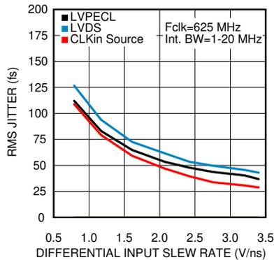
**Figure 7-15. RMS Jitter vs CLKIn Slew Rate at 625 MHz**
