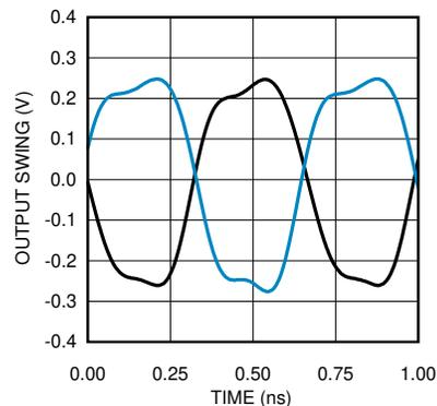
**Figure 7-6. LVPECL Output Swing at 1.5 GHz**
