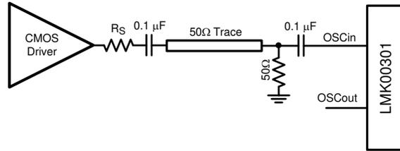
**Figure 10-4. Driving OSCin with a Single-Ended Input**
