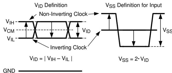
**Figure 8-1. Two Different Definitions for Differential Input Signals**
