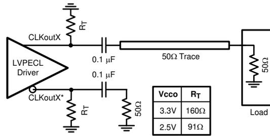
Figure 10-15. Single-Ended LVPECL Operation, AC Coupling
