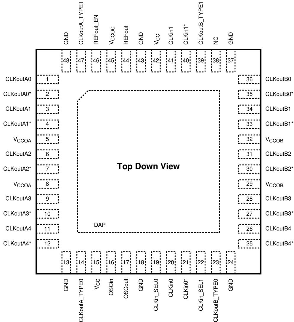
Figure 6-1. RHS Package 48-Pin WQFN Top View
