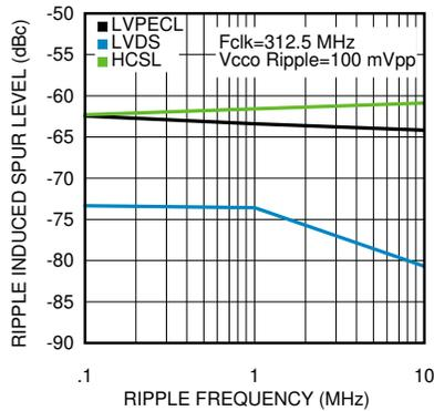
**Figure 7-17. PSRR vs Ripple Frequency at 312.5 MHz**
