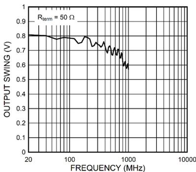
**Figure 7-3. HCSL Output Swing ( $V_{OD}$ ) vs Frequency**
