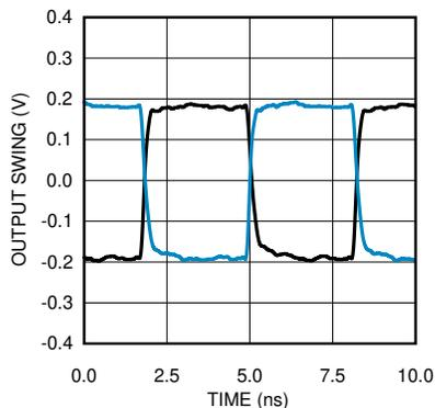
**Figure 7-5. LVDS Output Swing at 156.25 MHz**
