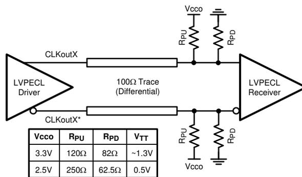
Figure 10-9. Differential LVPECL Operation, DC Coupling, Thevenin Equivalent
