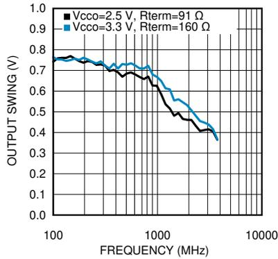
**Figure 7-1. LVPECL Output Swing ( $V_{OD}$ ) vs Frequency**
