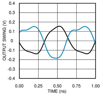
**Figure 7-7. LVDS Output Swing at 1.5 GHz**
