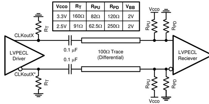
Figure 10-12. Differential LVPECL Operation, AC Coupling, Thevenin Equivalent
