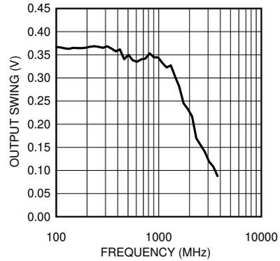
**Figure 7-2. LVDS Output Swing ( $V_{OD}$ ) vs Frequency**
