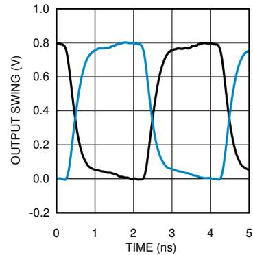
**Figure 7-8. HCSL Output Swing at 250 MHz**
