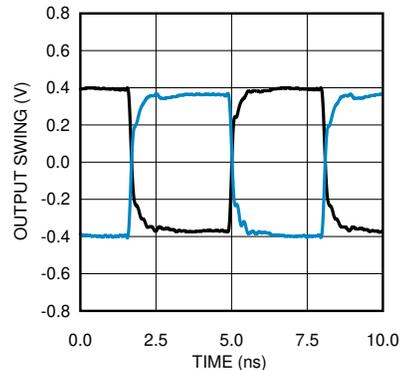
**Figure 7-4. LVPECL Output Swing at 156.25 MHz**
