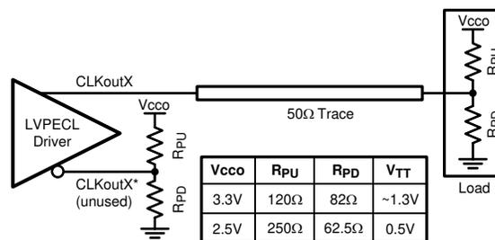
Figure 10-14. Single-Ended LVPECL Operation, DC Coupling, Thevenin Equivalent
