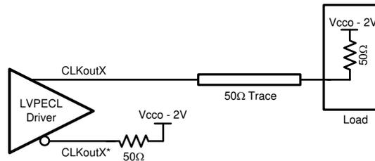
Figure 10-13. Single-Ended LVPECL Operation, DC Coupling
