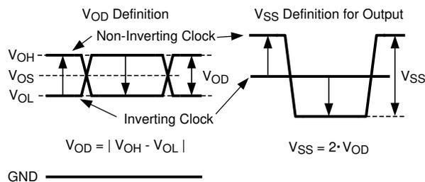
**Figure 8-2. Two Different Definitions for Differential Output Signals**
